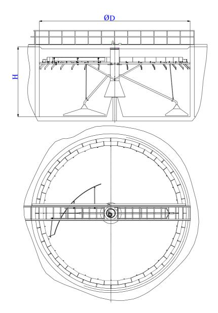
Inclination of the bridge: L/200, L/400
