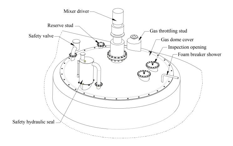
The material of the armatures and of the tank cover is made of anti-corrosion steel.
